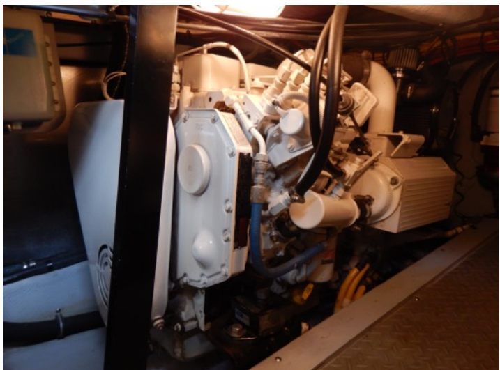
Twin Diesel Powered 250HP CUMMINS Inboard Engines w/ ZF HURTH Straight-Drive Reduction Gear Transmissions
